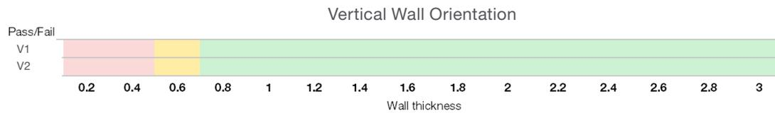
**Table 1:** Red designates a complete failure to build, yellow designates a passing build with significant inaccuracies, and green represents a complete build for each wall thickness.
