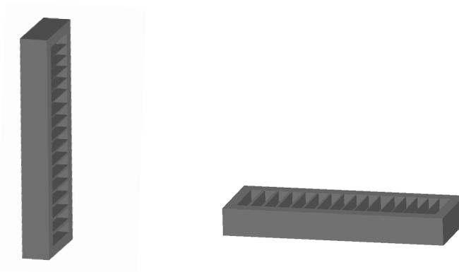
**Figure 1:** Via the left side orientation, the walls are horizontal with relation to the surface of the build where the build top is located at the uppermost surface; therefore this orientation will be referred to as the horizontal orientation. Via the orientation shown on the right, the internal walls are vertical in relation to the surface of the build therefore this orientation will be referred to as the vertical orientation.
