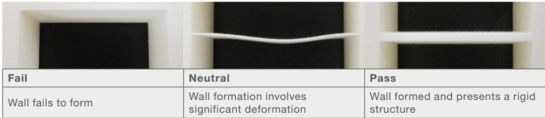
**Figure 2:** Pass/ fail criterion for external wall thickness/ thinness.
