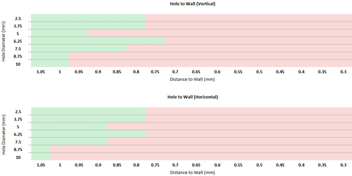
**Table 3:** Pass/fail matrices for hole diameters and distance from other features (in this case, the edge or wall of the part).
