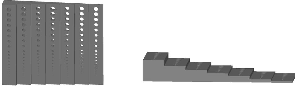
**Figure 3:** There are 21 holes per step with diameters ranging from 0.125 mm to 4 mm. In the orientation shown to the left, the hole features are horizontal with relation to each Z-axis cross-section therefore this orientation will be referred to as the horizontal orientation. The image on the right shows the hole features in a vertical orientation in relation to each Z-axis cross-section therefore this orientation will be referred to as the vertical orientation.
