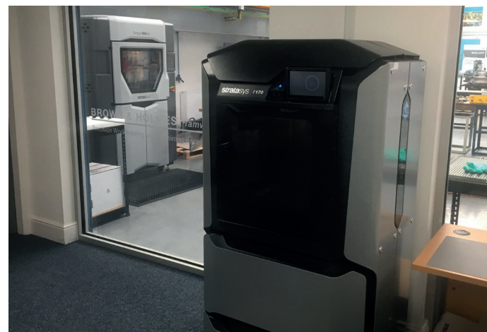
The Stratasys F170 is used to print elastomers, while the Fortus 450mc produces high performance materials that can withstand very high temperatures
