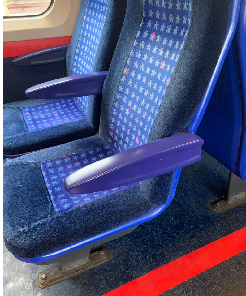
3D printed armrest on Chiltern Railways train – produced 94% faster compared to traditional manufacturing methods.
