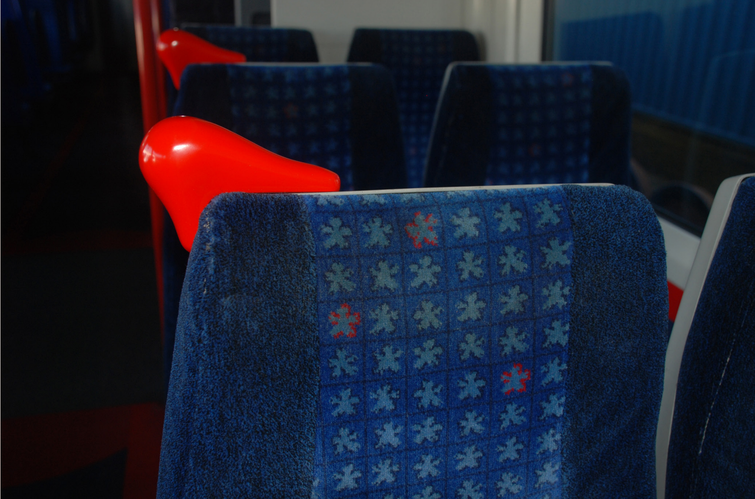
3D printed grab handles installed on a Chiltern Railways train.
