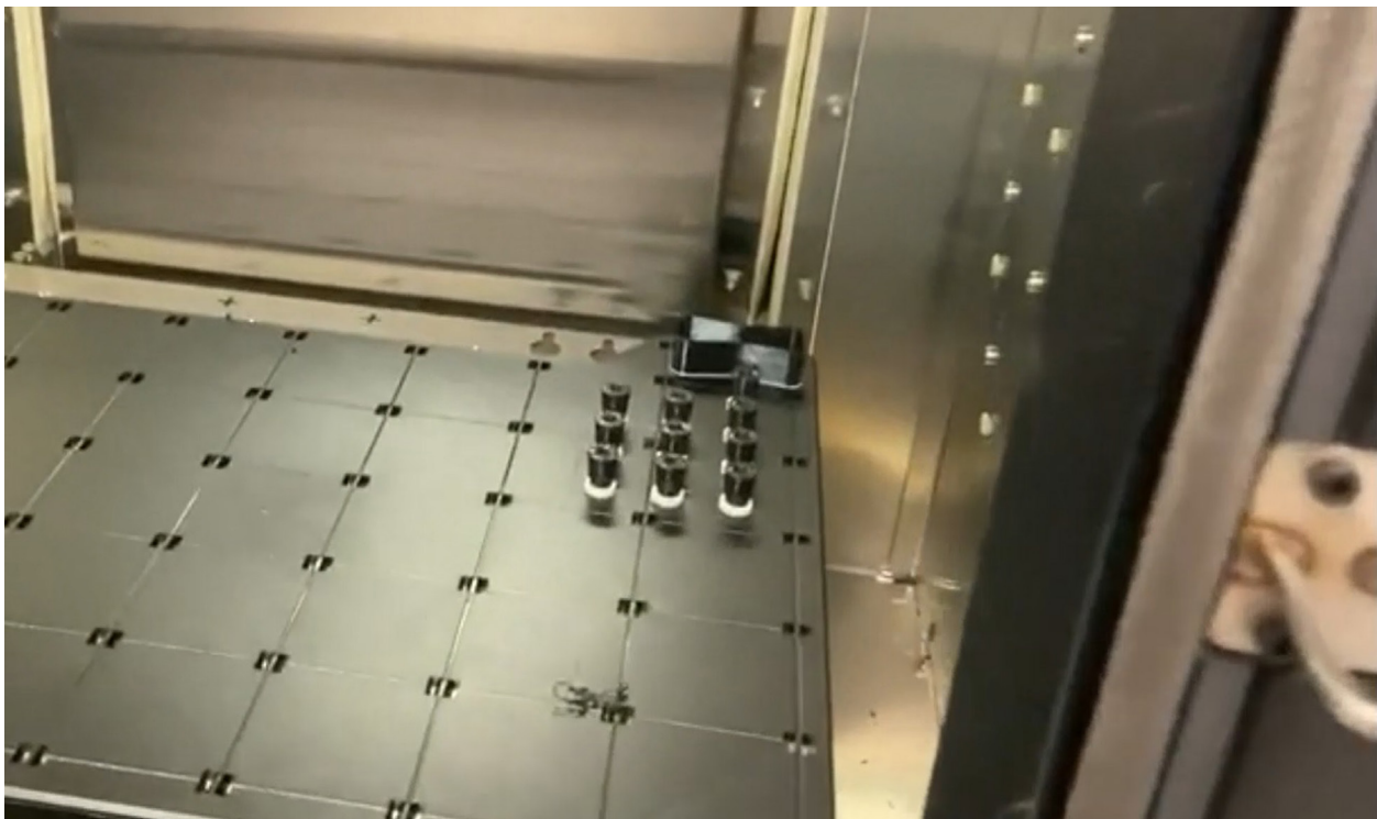
Using Stratasys FDM 3D printing, Alstom was able to design, produce and deliver a dozen highly durable stoppers within just 48 hours of receiving the request from Sétif.
