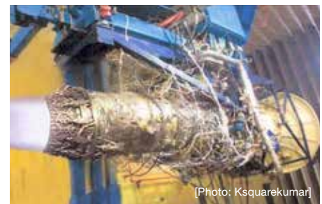
The Kaveri engine prototype on a test-bed. [Photo: Ksquarekumar]
