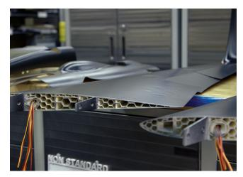
Internal wing design, optimizing complex internal structures, for lightweighting aircraft.
