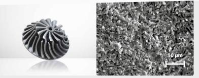
SILICON NITRIDE is a Beta-SiAlON type ceramic. It exhibits superior material properties such as **high strength**, high **toughness**, **thermal shock resistance** and good **chemical resistance** to corrosion by many acids and alkalis. It is well suited to applications in the **medical** field and those which require high **thermal resistance**, as well as for use as cutting tools.
