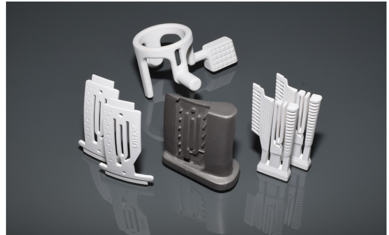
Fig. 3 Investment casting cores manufactured from silica-based LithaCore 450 after printing and sintering, along with a cast metal part. The cores were produced on a CeraFab 8500 printer (Photo Manfred Spitzbart)
