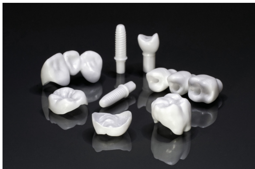
Fig. 5 In dentistry, LCM allows for the production of full ceramic crown, ultra-thin occlusal veneers for minimal invasive reconstruction and endosseous screw-type dental implants. Fine edges down to 100 \mu\text{m} can be achieved
