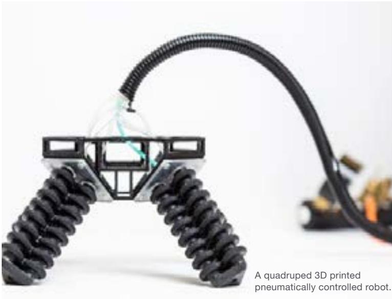
A quadruped 3D printed pneumatically controlled robot.
