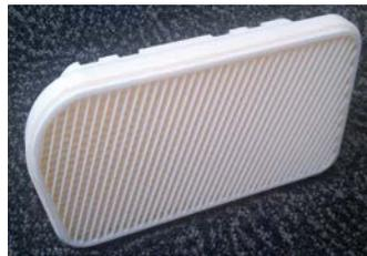
FDM paper pulp tool with custom sparse fill
