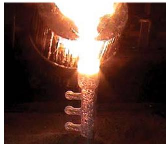
Pouring metal into gear set casting shell.
