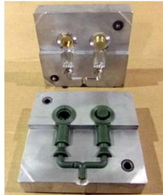
Typical example of aluminum injection mold and wax pattern.
