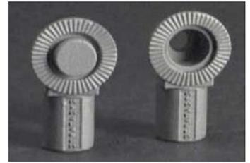
For RLM Industries, investment castings were produced to specifications in only seven days using FDM method.
