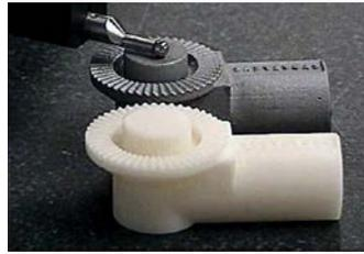
Male FDM pattern (foreground) and finished casting being inspected with coordinate measuring machine touch probe.
