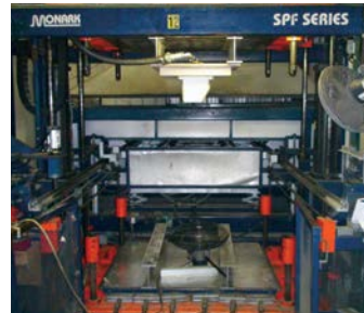
FDM tool mounted in thermoforming machine
